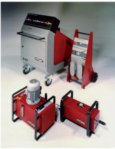
HYDAC nitrogen charging units facilitate fast and cost-effective charging or testing of the required pre-charge pressures in bladder, diaphragm and piston accumulators. They guarantee optimum use of standard nitrogen bottles up to a residual pressure of 20 bar and a maximum accumulator charging pressure of 350 bar. Portable, mobile and stationary types of  $N_2$ -Server are available.
