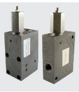
HYDAC accumulator charging valves control, within an adjustable switching range, the charging of the accumulator. By combining the charging valve with an accumulator, pumps and motors on hydraulic plants with fluctuating flow requirements can be sized smaller. This saves costs and energy - thus preventing unnecessary heat development.
